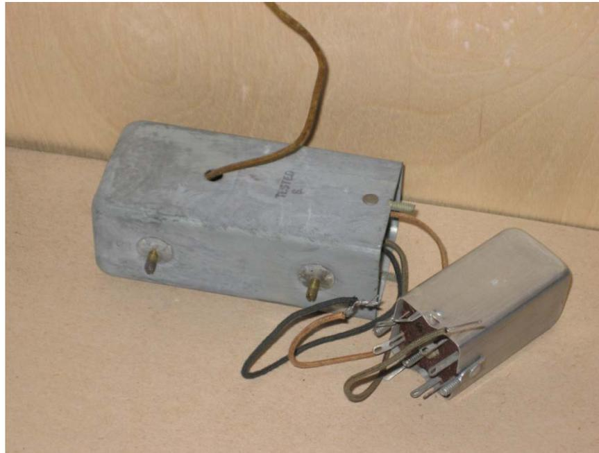
These are usually (but not always) in shield cans, which help keep stray radio interference signals from entering these high-gain stages.
