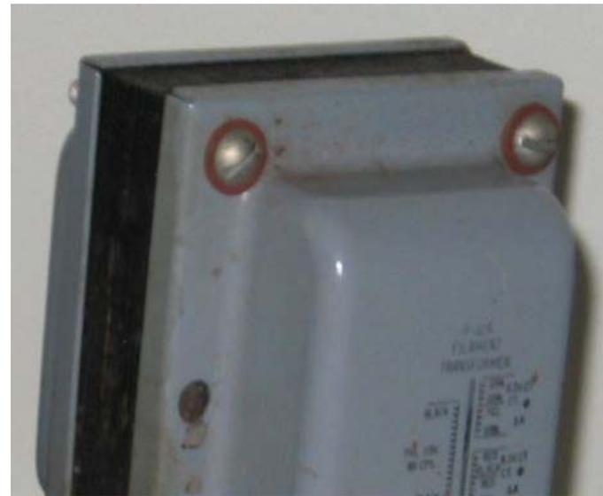
Many have shells held in place by the bolts at the corners. Here we have one in which the bolt-heads are insulated by fiber washers; not so with the other.
