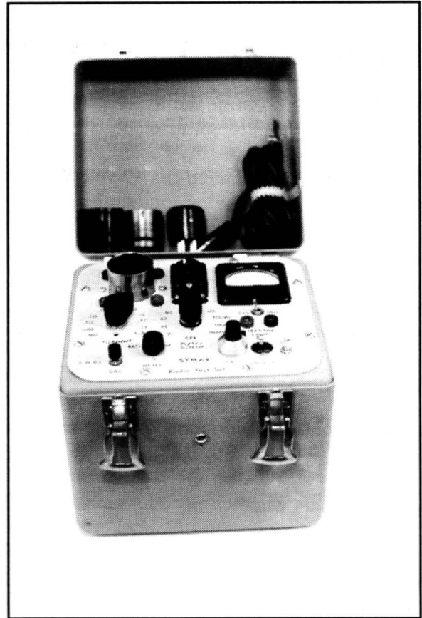
Figure 1. The tube tester in its carrying case, with adapters and test leads in the lid.
