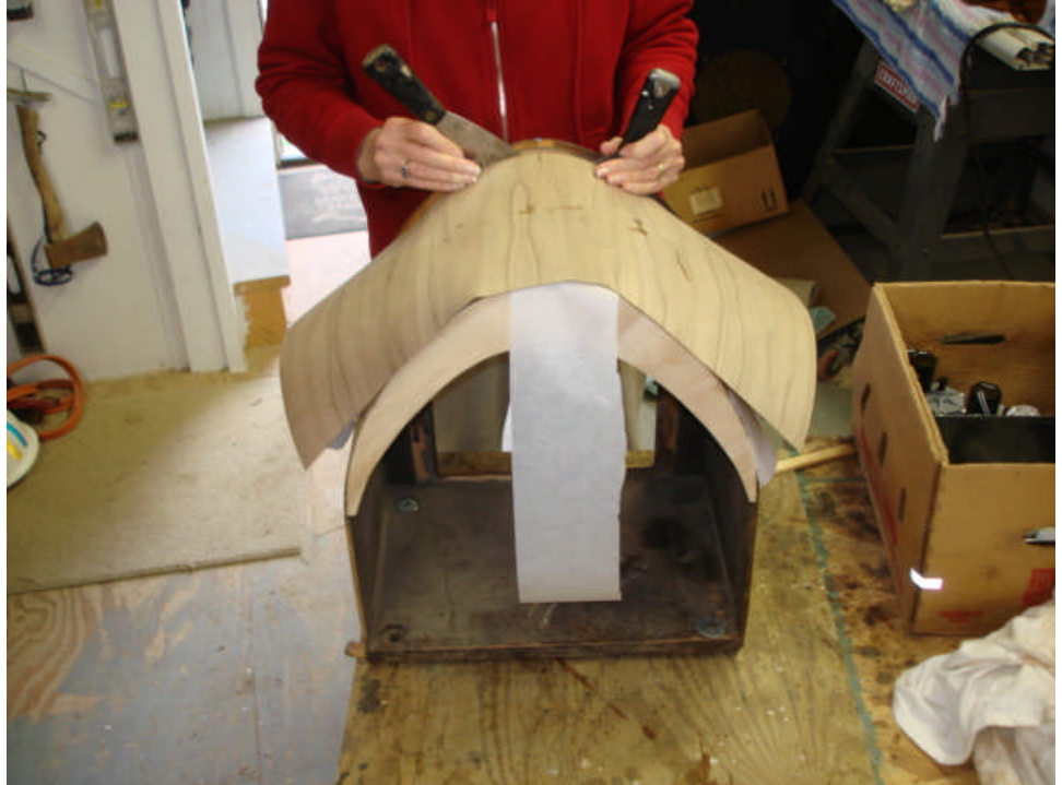
Here I am beginning to attach the new veneer to the top of the cabinet.
