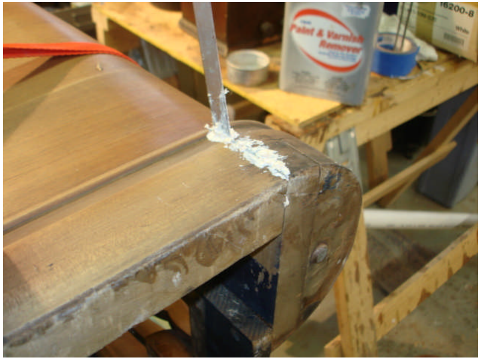
Securing a loose joint in the base of a cabinet. Force the glue-sawdust mixture in with a thin tool.
