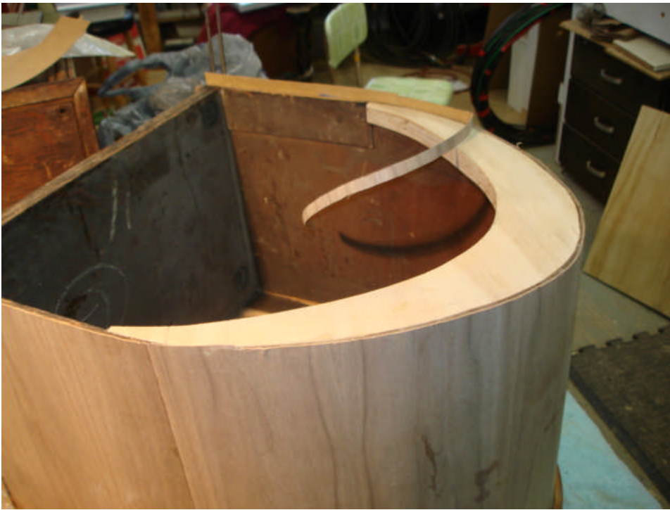
Trimming the excess veneer from the rear of the cabinet.
