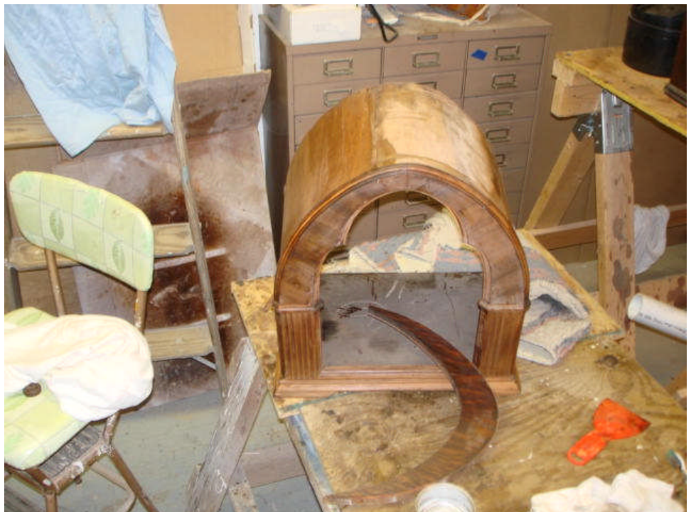
The arch at the top rear of this Philco 90 cabinet needed to be replaced.
