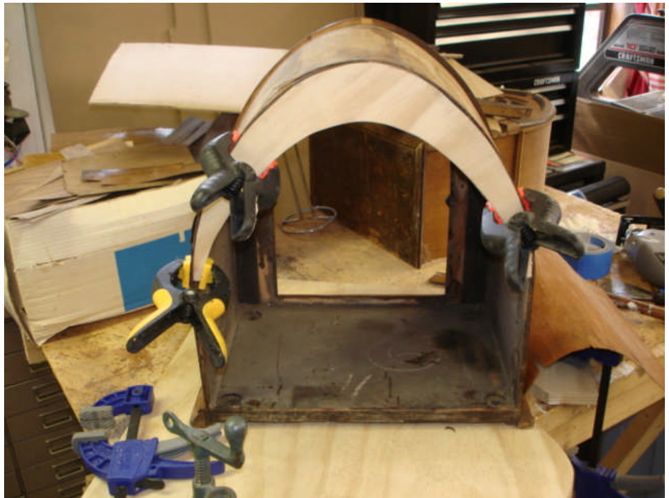
The replacement arch is now firmly attached to the top of the cabinet, using tiny nails through the sub veneer.
