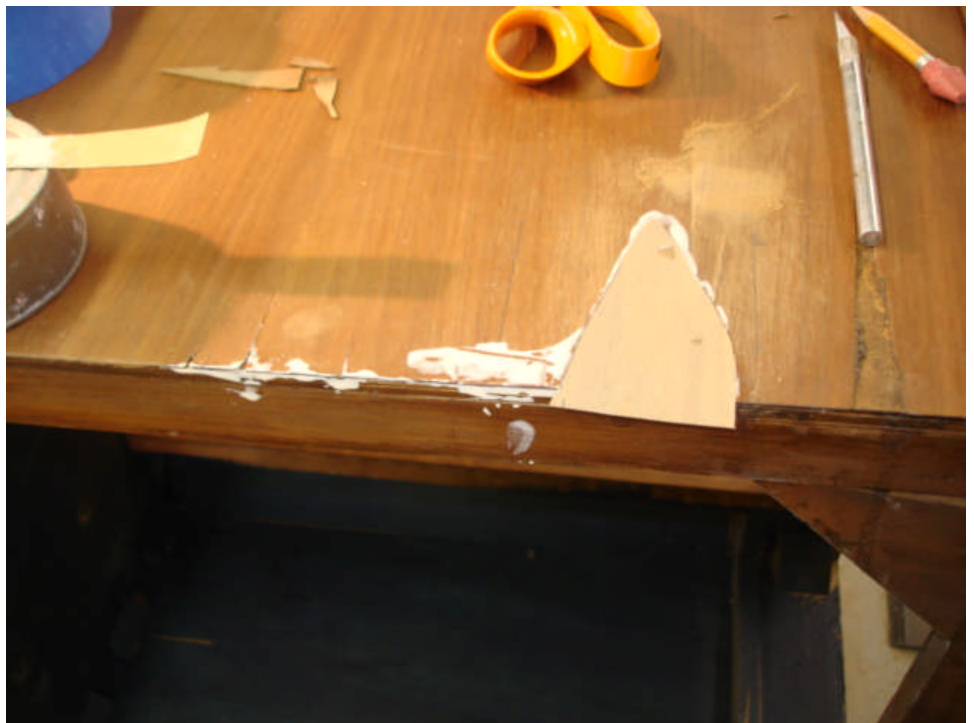
This Zenith cabinet needed veneer patches. Here I apply a piece of scrap veneer larger than the damaged area and then cut through both pieces with the Exacto knife.
