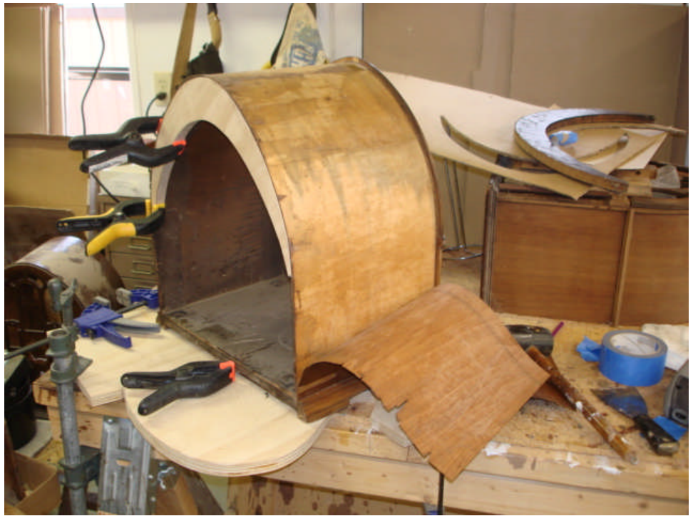
In this photo the replacement arch is being fastened to the top of the cabinet.
