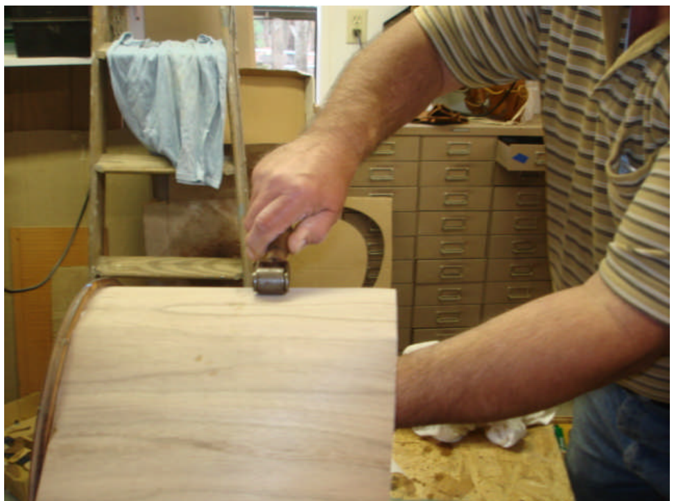
Rolling the veneer to eliminate air bubbles between the glue and the veneer and ensure a tight bond.
