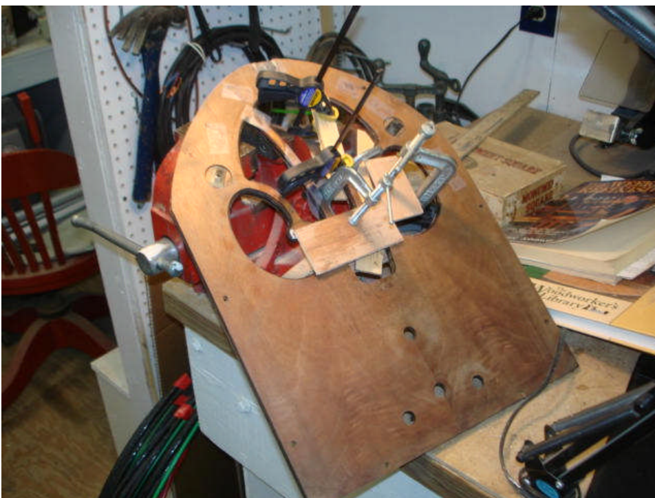
Repairing the grille. Here again, it is essential to have enough small clamps on hand.
