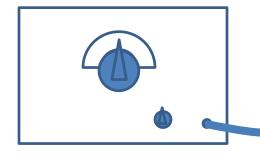
Set signal generator to, say, 455+800 kHz (1255 kHz) with modulated signal, high strength. Lay the coil on the dead transistor radio. Search for this signal with dead radio dial around 800 kHz. If it comes in, the full audio section is working, Thus either the IF amplifier or LO is inoperative.
