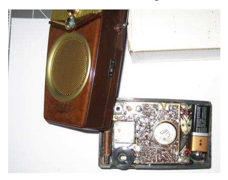
Here, we use a little Philco AM-FM set to create a LO signal for the broken radio. Sweep the LO frequency through the 1255 kHz region, with the good radio's gain at minimum, and the broken radio's gain at maximum.
