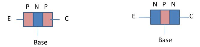
NPN transistors operate primarily by movement of Electrons, instead of Holes, and can be much faster in response, suitable for UHF, for example.
