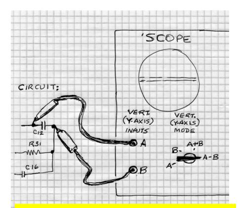
Any a-c signal showing on 'scope means that the electrolytic cap is dried out. If the expected d-c voltage does NOT show up, the cap may be shorted.
