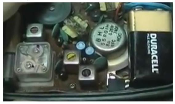
You confirm that the battery in it is good, and that the battery voltage gets to the circuit board, which checks the 9-volt battery's plug-in snaps and the wires from that to the circuit board. This also checks that the on-off switch on the volume control seems to work.
