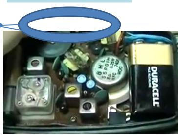
But a fast way to do this, without having to get out the signal generator, is to use another small transistor radio, in working order, to create or detect signals. Its LO will generate a signal that's 455 kHz above the dial reading, Set both radios to about 800 kHz dial settings.
