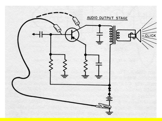
This is, generically, how to use the "clicker." In the radio at hand, the output is push-pull, so you would do this for both output transistors and for the driver, also transformer-coupled to the output pair.
