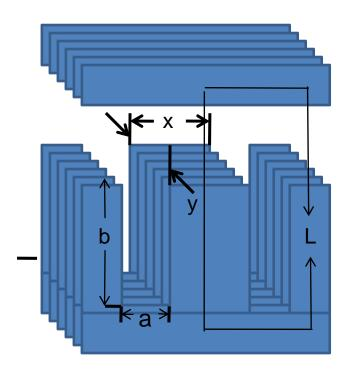
The window size determines how much power we can get, for a given core area. It actually determines how much wire of a given gauge can be stuffed through the windows.
