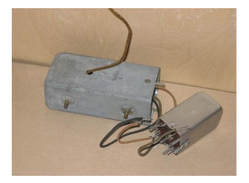
These are usually (but not always) in shield cans, which help keep stray radio interference signals from entering these high-gain stages. The two IF transformers here are not identical to each other. In better radios, the output IF "can" has a lower impedance secondary because it has to feed a load (the detector diode and volume control, for example)'
