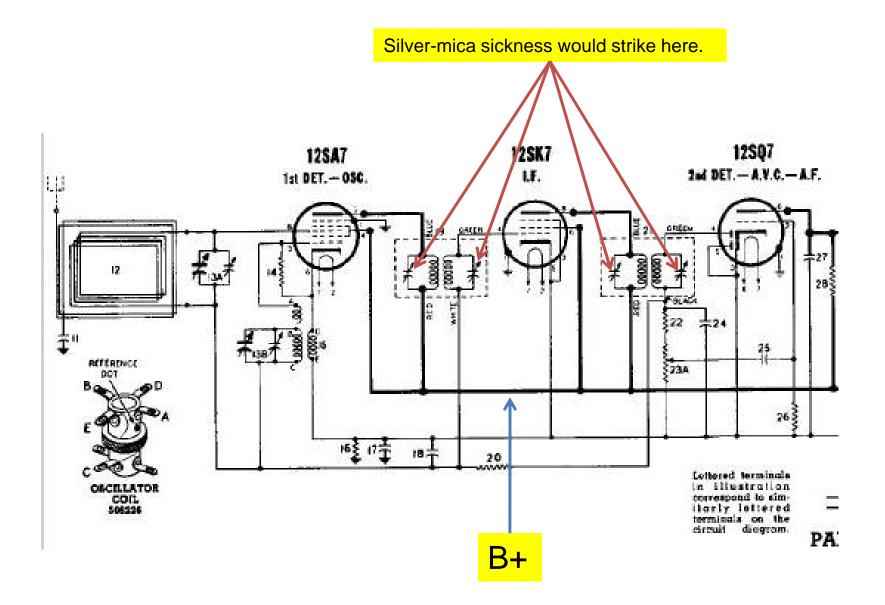
Power transformers and audios fail due to the voltages present and the currents they carry, which are usually sufficient to promote electrolytic corrosion and/or heating, which results in expansion and contraction with periodic use. Having no core gap, they are unforgiving if a secondary winding has a load that gets short-circuited, like a failed electroilytic cap in the B+ line, or a shorted audio output tube's plate-to-ground capacitor.
