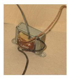
120-to-6V power Xformer Plate-to-v.c audio Xformer \* The miniscule gap in the core of the audio transformer provides sufficient permeability reduction to "absorb" the voltage spikes in audio without saturating the core. And, then there are I-F transformers (or "cans") used in interstage coupling in I-F amplifiers and in discriminator stages in FM or PM circuits.
