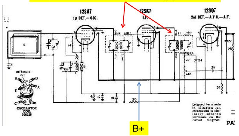
The primary advantage of superhets is that most of their amplification of radio signals takes place at a primarily fixed frequency, the I.F. This allows optimization of the I-F transformers rather than live through the compromises in designs of RF transformers (e.g., the AM B-C band spans a 3:1 frequency spread).
