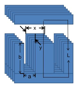
In the type of core shown, L is the magnetic path length and (a) times (b) is the window area, which must hold all the wire turns.
