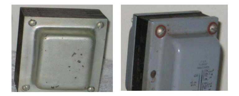
Many have shells held in place by the bolts at the corners. Here we have one in which the bolt-heads are insulated by fiber washers; not so with the other. Other shell-type power transformers use side-mounting bolts and slotted passages in the laminated core for these bolts. These transformers have fewer hum and corrosion problems than those with corner bolts.
