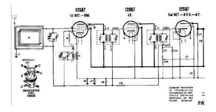
And an E.H. Scott multiband set. Note each band uses its own RF transformer rather than try to use a tapped multi-band winding.
