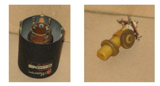
Note the rather loose coupling between primary and secondary on the one on the right.
