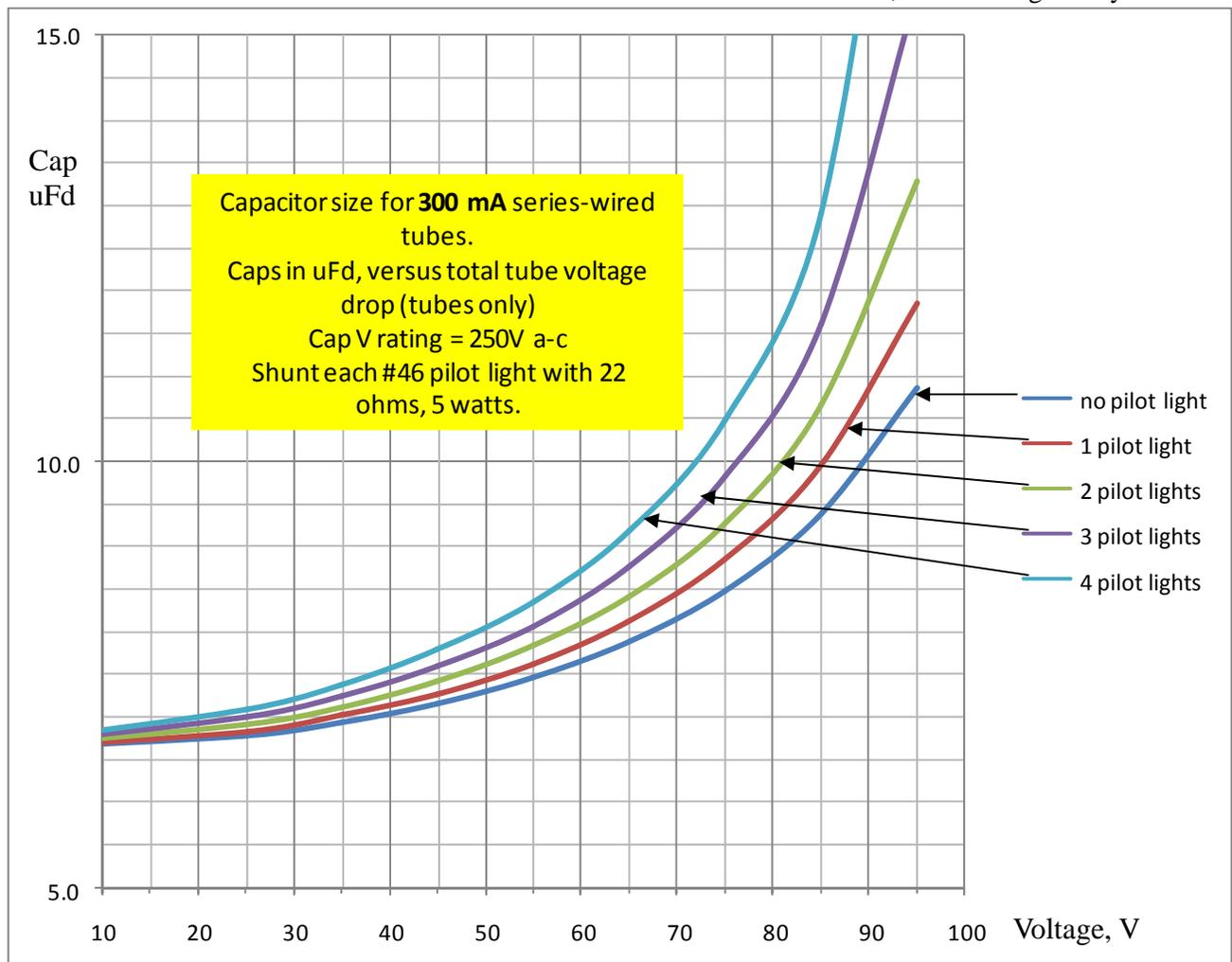
For those more rare cases where there is a 150 mA tube string, like 35L6, 35Z5, 12 SA7, etc., etc., there is a similar chart on this page. Difference here is that you would use type 47 bulbs practically all the time, but in a few radios, screw-type bulbs are called for, which means you use type 40 bulbs, and now, with all bulbs in 150 mA tube strings, you shunt the bulb terminals with a 22 ohm, 2-watt resistor.
