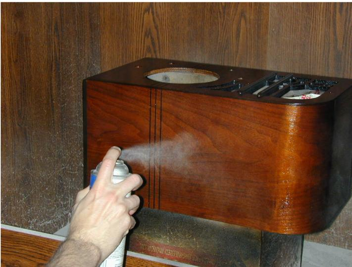
**Figure 17: Spraying the clear coat.**
