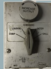
BC-366 jack box, with volume control and several channels selectable by the crewman
