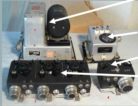
Dynamotor to Power the Transmitters & Modulator BC-456B
