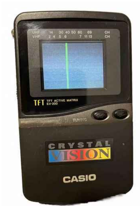
Casio TV EV-200B with auto tuning. The green (UHF) scan line suggests a working set.
