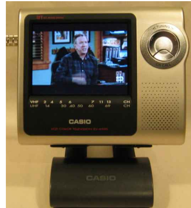
Casio EV-4500 (2003) 4 in. color LCD TV. Thin film transistor (TFT) active matrix screen. 122,920 pixels. Digital tuning.
