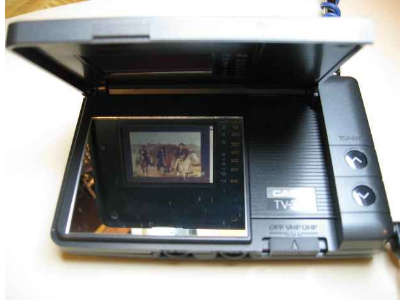
Indirect-view LCD. Casio TV-300. (1986). Snap-on backlight panel was an optional extra.
