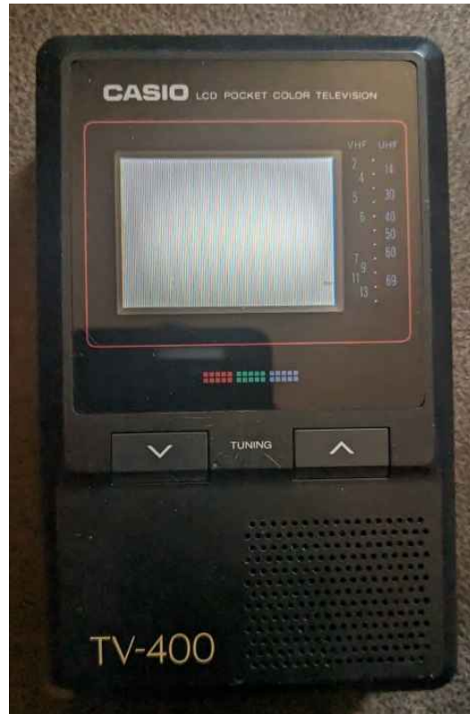
Casio TV-400 LCD TV with auto tuning. The snowy screen and visible channel indicator tab suggest a working set.
