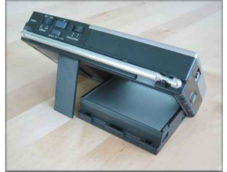
Hybrid light source. Epson ET-10 LCD TV (1984). Reflective panel can be pivoted into or out of position.
