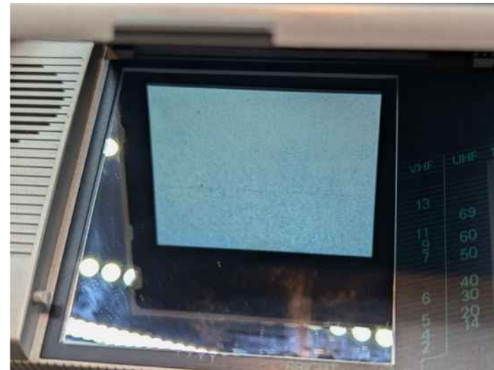
Citizen TV-06TA B&W LCD TV indirect view set. Manual tuning. The mirror shows the screen has a full raster with snow throughout the screen.
