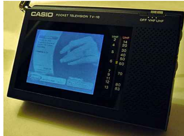
Casio TV-10 (1983). World's first self-contained LCD TV. (Visions4 magazine – Page TwoA).
