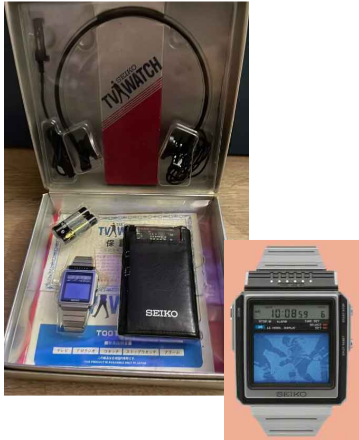
Seiko T-001 TV Watch (1982). World's first device with LCD TV screen; 1 ¼ inch . (e-bay; and www.seiko-design.com/140th/en/topic/51.html )
