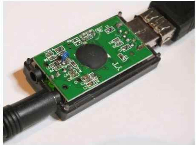
E-Panorama brand USB-connected 'scope adapter for laptop.
