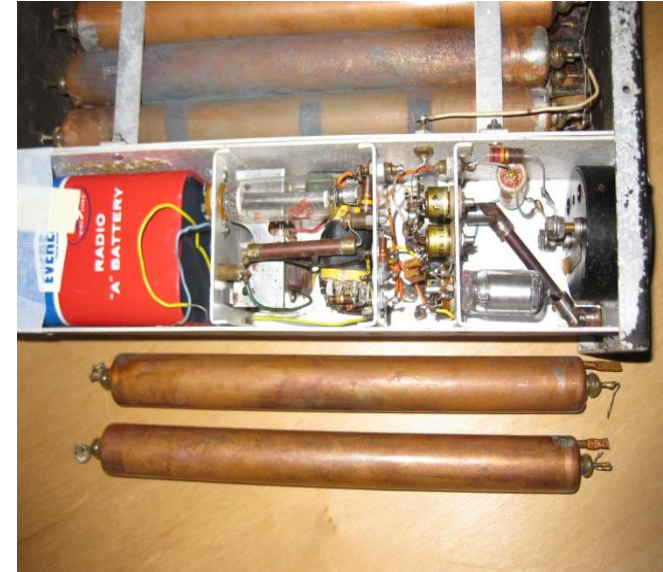
NRL's Neutron counter, made for the Manhattan Project, 1942-44
