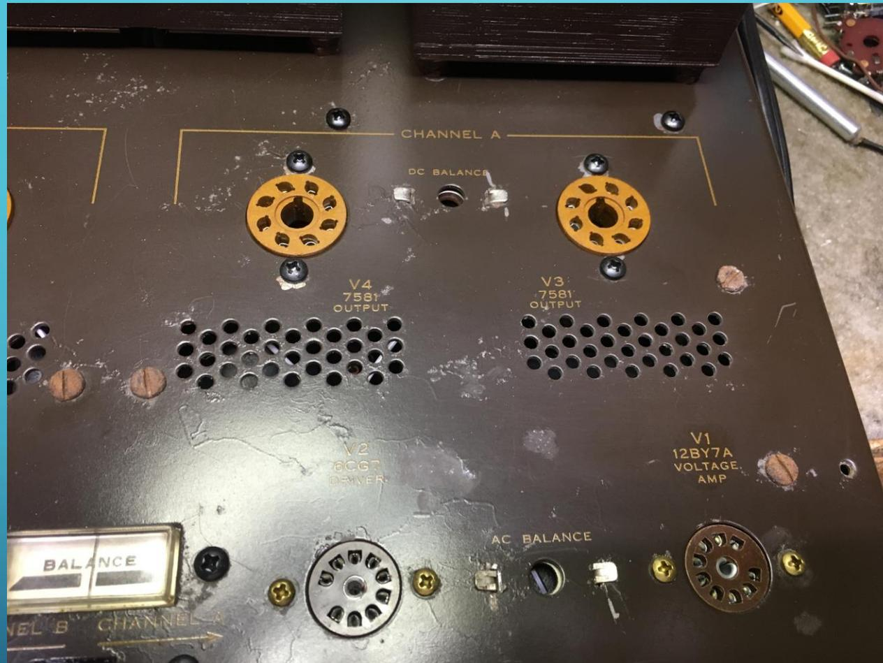
Note the screw heads here, these are the original which will be replaced but gives an indication of the degree of corrosion of this unit before restoration
