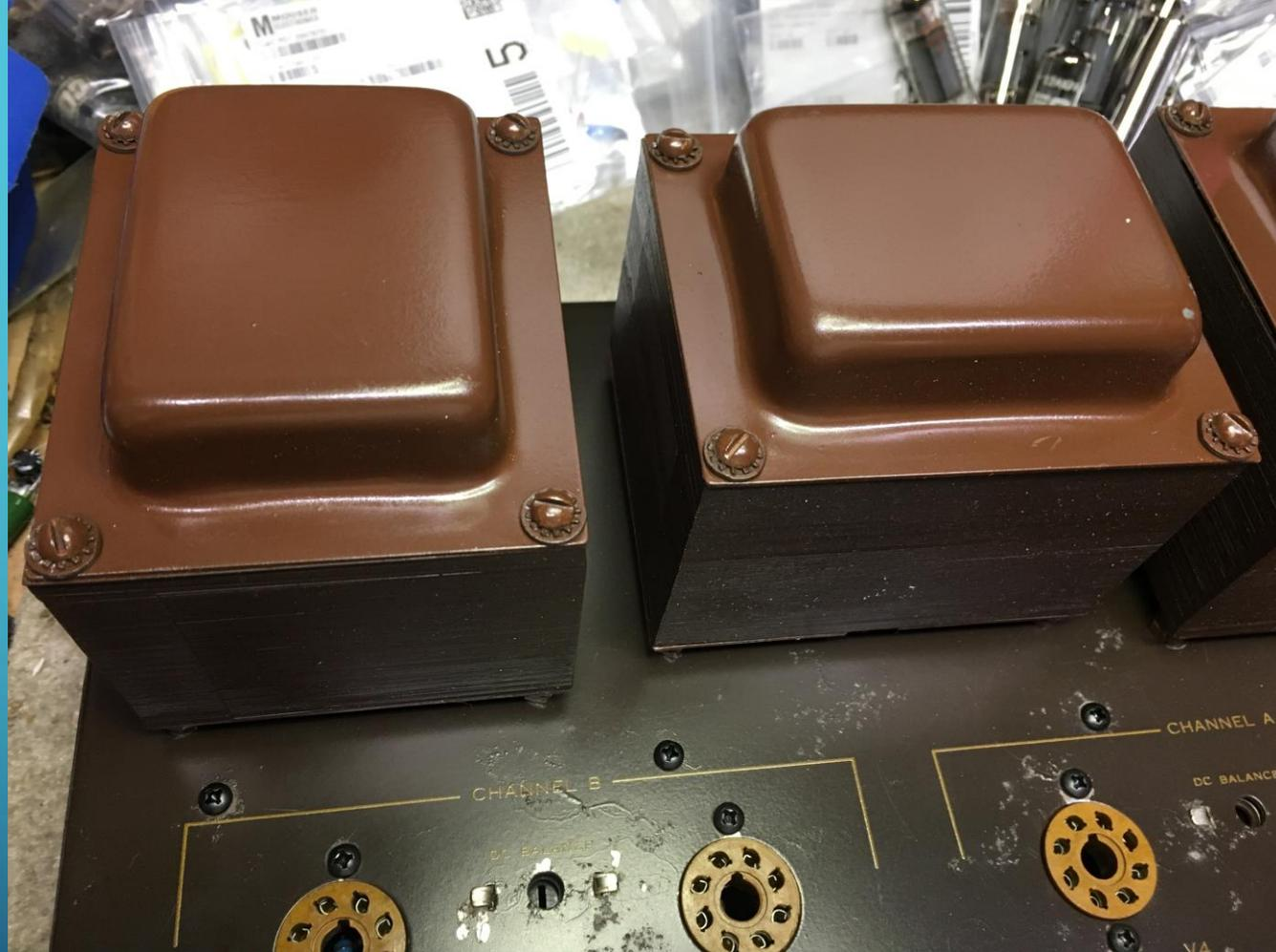
Note the repainted transformer bells and lams, also the buffed chassis
