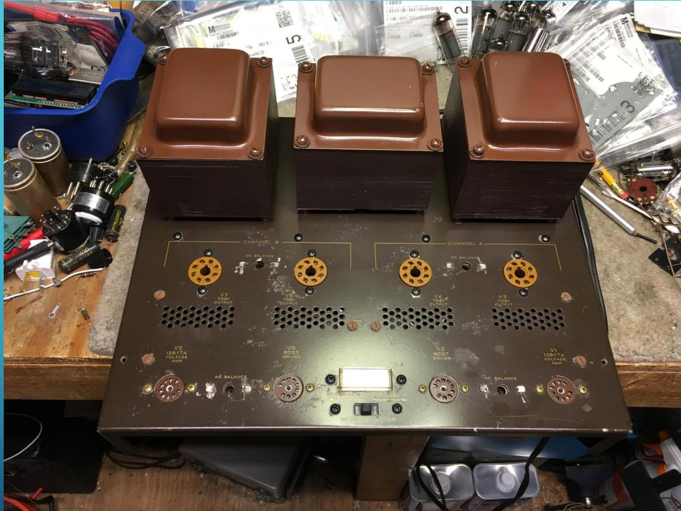
Noted is the new tube sockets and the repainted transformers which were rusted
