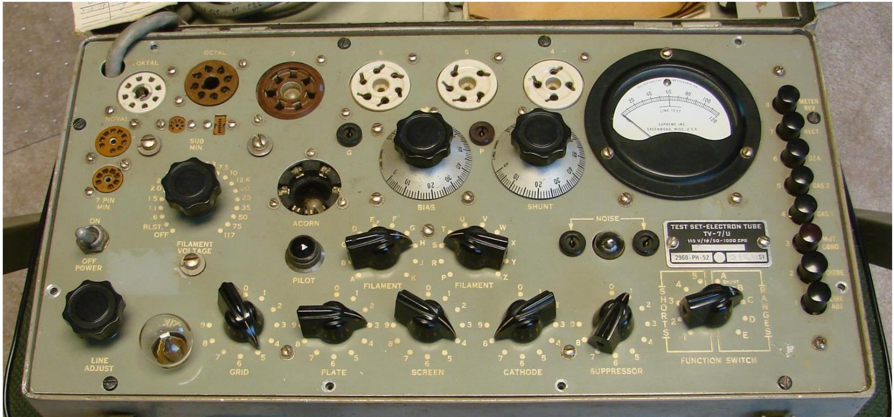
**Note the skirted dials on the Bias and Shunt controls. Later variants had number settings engraved in the panel. Except for the first Navy run by Hickok in 1952, all U's were made by Supreme Instruments, company bought by Hickok in 1956.**
