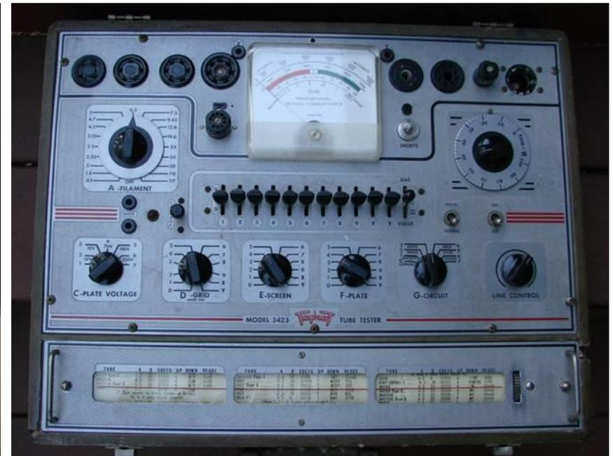
Both versions identical electrically in the gm test - “Proportional Transconductance”
