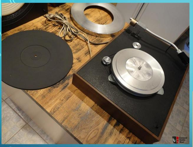
AR XA turntable showing belt mechanism and underside spring mounting
