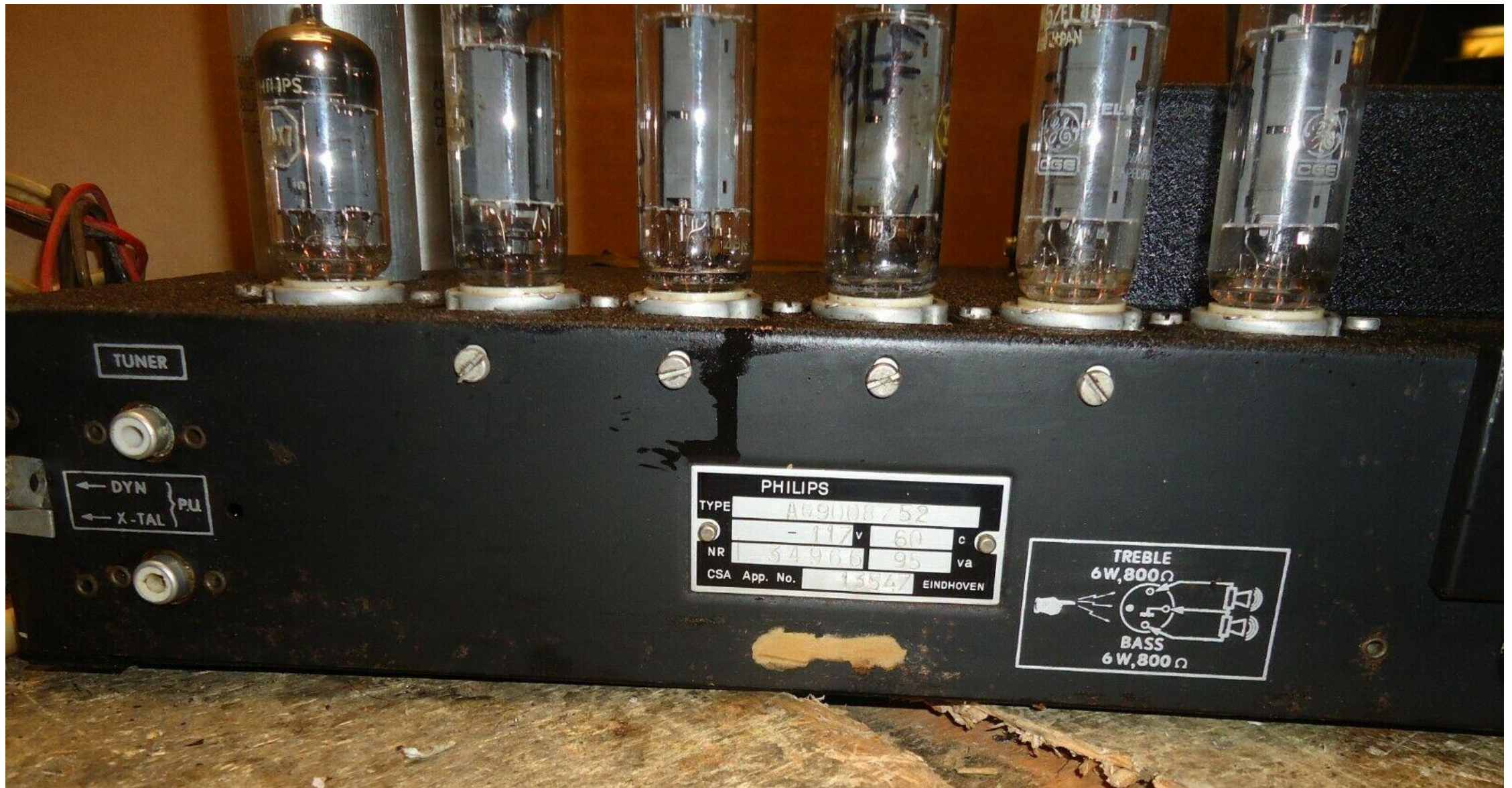
Philips Hi Fi OTL amp for high-impedance speakers CIRCA 1955 , MADE IN EINDHOVEN HOLLAND
