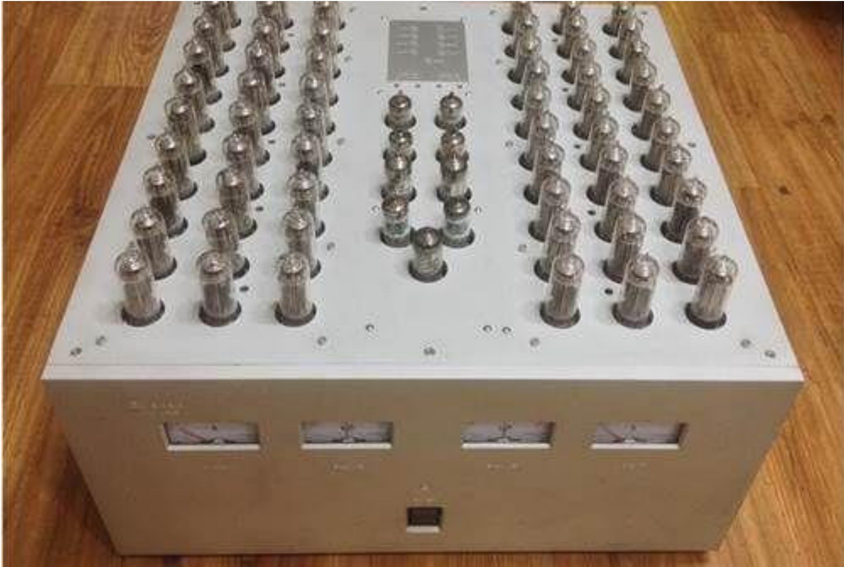
Silvaweld OTL Reference 200, 30 output tubes per channel.
