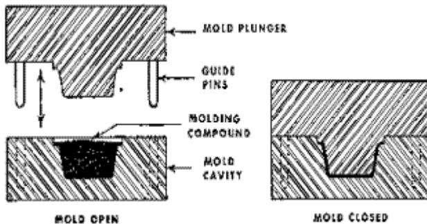
The mold is often made of heavy steel interlocking parts, so that it can be disassembled to remove the product, and yet is strong enough to withstand the molding pressure. Upon removal from the mold, the cabinet is completely finished, needing only a quick once-over to remove the paper-thin "flash," remnants of resin that have oozed into microscopic seams between parts of the steel mold.
