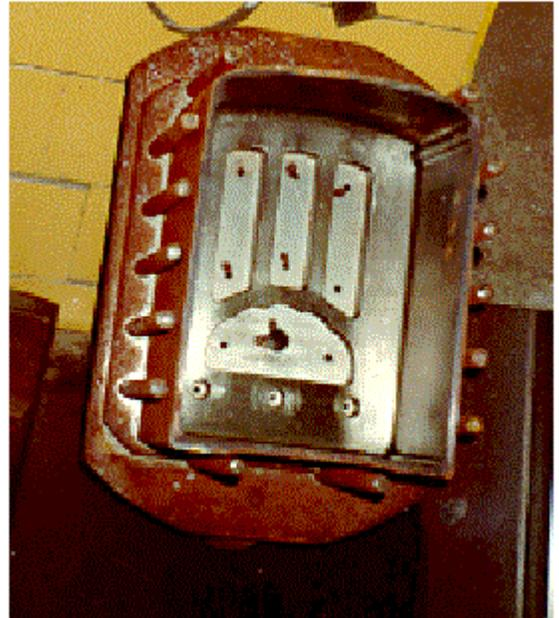
The arbor is highly polished (not rusty like the one in the figure), with a large handle on its topside, which is the flat plate forming the “front” of the radio cabinet. It weighs perhaps 80 pounds, so it is lifted, using its handle, by a hoist system, using chains or cables. It is swung over a heated vat filled with melted lead, and suddenly dunked into the vat and quickly withdrawn. A coating of lead freezes in place on the arbor, which, with the lead coat, now weighs perhaps 130 pounds.
