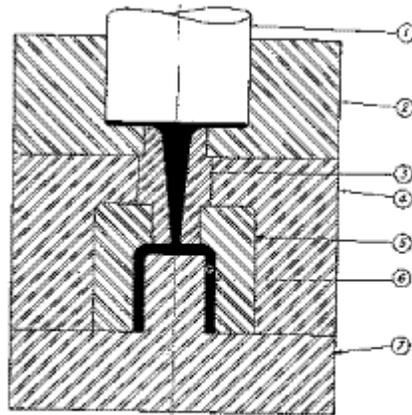
Fig. 2-11. The "integral" or "accedion" type of transfer mold.
