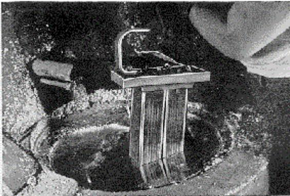
An example of an arbor being lead-dipped can be seen at the left, the picture taken from a pre-war text on plastics. The lead-clad arbor is then slammed downward between two anvils which catch the outboard portions of the extended plate forming the radio front. The lead coating slides off the arbor, and is caught in a padded base between the anvils, so that it is not damaged. Now, the lead has a cavity in it, exactly the shape and size of a radio cabinet.
